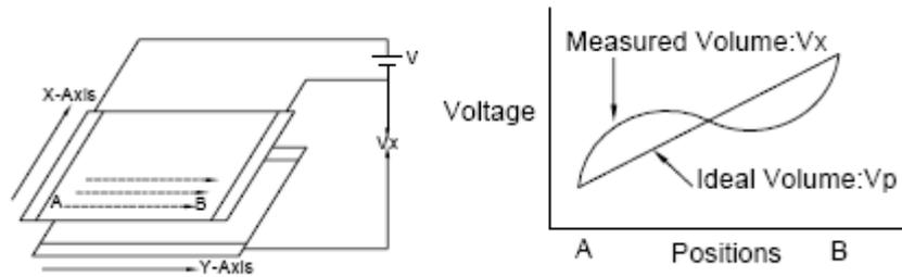
$$\text{线性} = | \{ (V_p - V_x) / (V_a - V_b) \} | \times 100 [\%]$$
